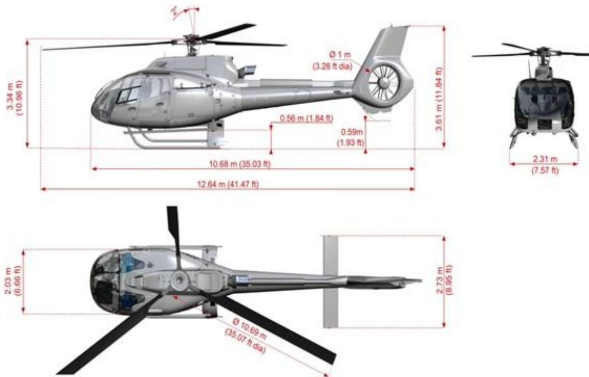
Photograph # 2: Primary dimensions of the helicopter H130
