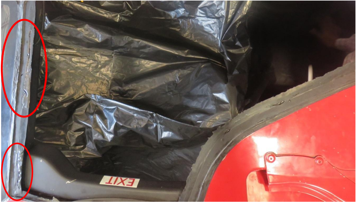
Photograph # 7: Uneven surface & Lumps found on periphery of adhesive area
